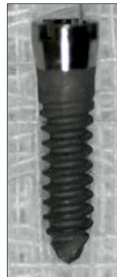
Fig 1 The implant used in this study (C-implant). It comprised two parts: a 6.5-mm SLA surface screw part and a 2-mm smooth-surfaced transgingival part. The diameter of the implant was 1.8 mm.
