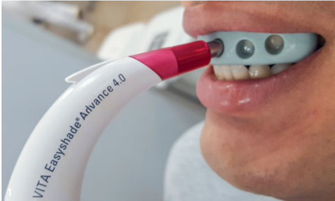
Fig 1 Silicone guide with the tip of the Vita Easyshade spectrophotometer to standardize color selection.
